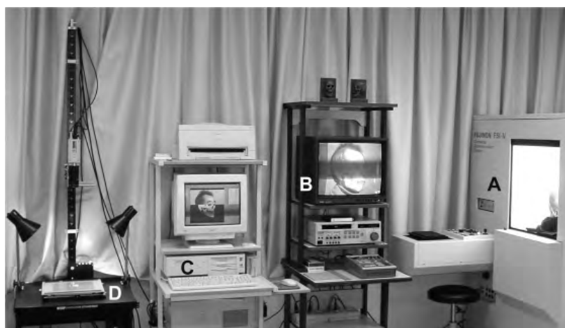
Figure 19.1 Computer-assisted skull identification system using video superimposition. A: Skull-positioning box; B: Video superimposition unit; C: Computer-assisted skull identification unit; D: Photo-stand for facial photograph. The skull position is moved in any direction by remote control lever using the pulse motor-driven mechanism.
